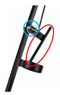
To make adjustments to the trigger system, simply unpin the clip (circled in blue) and swop to the other end of the bar (circled in red).
